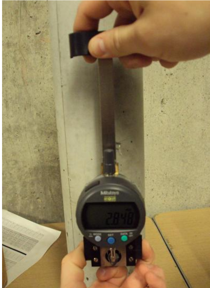
Figure 3.3 – DEMEC Reading Taken on Specimen
