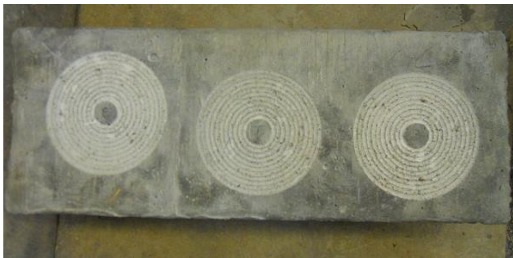
Figure 3.15 - Abrasion Resistance Specimen After Testing
