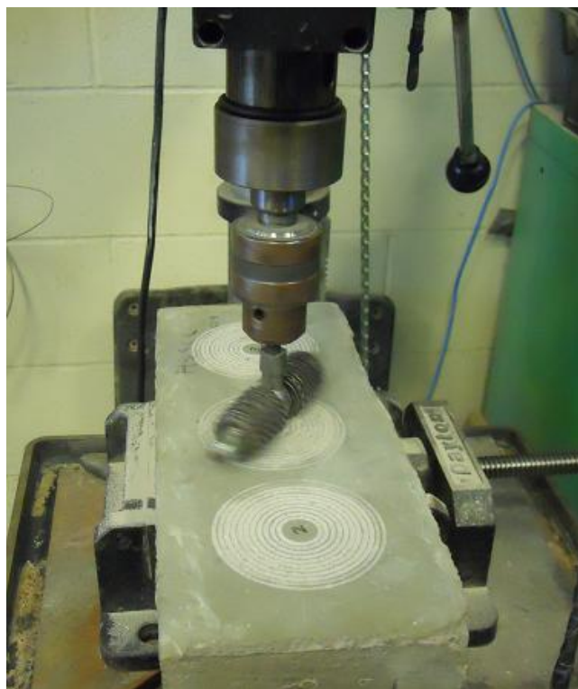
Figure 3.13 - Abrasion Resistance Test In Progress
